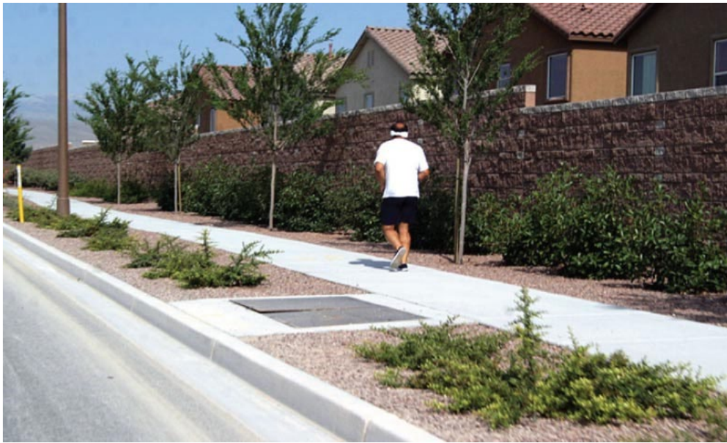
Figure 3-1. Five-Foot-Wide Sidewalk with Buffer Example
